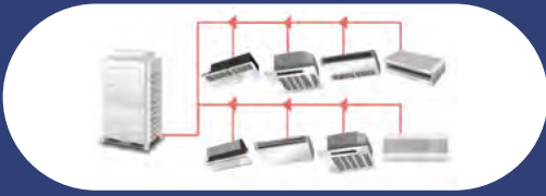
Variable Refrigerant Flow System
