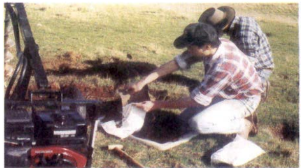
Collecting soil samples using a power auger
